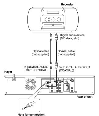
Remove the protection cap from the cable.
